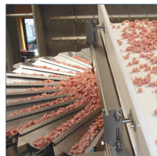
The conveyor loading the Linear Drive radial feeders
